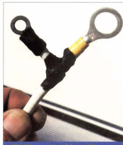
Maritime and vehicle mobile coax connections need to be waterproofed with Coax Seal™.
