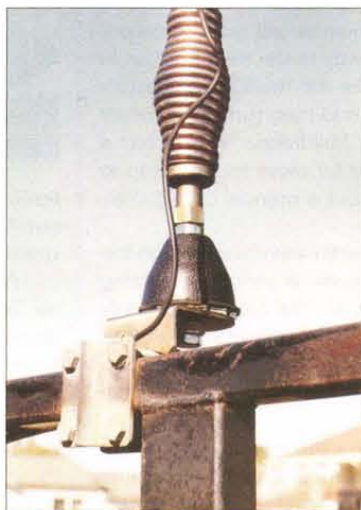
RV mounting of the quarter-wave whip on top of roof rack.
