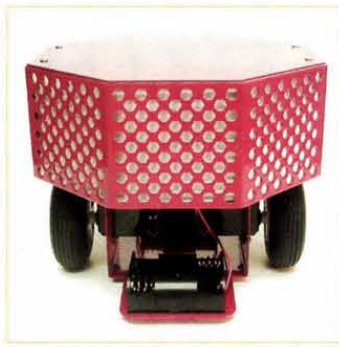
Figure 4. Expand the EasyBot (EasyBot/Michael Berta Ent) motorized base with a microcontroller and other electronics.
