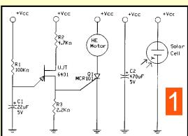
can stack low-voltage solar cells in series to reach a usable (2-2.5 volts) voltage, one should not add solar cells to increase the current. There's a reason for this: In order for the circuit to recycle, the current through the SCR must stop (or at least be very minimal), for the SCR to close. If there is too much current supplied by the solar cell(s), the SCR will stay turned on. If this happens, the circuit will stop cycling.
