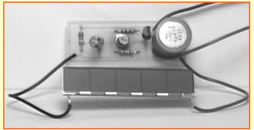
The solar engine circuit is simple and non-critical. It may be constructed using point-to-point wiring on a prototyping breadboard. A PCB pattern is also included for those who want
