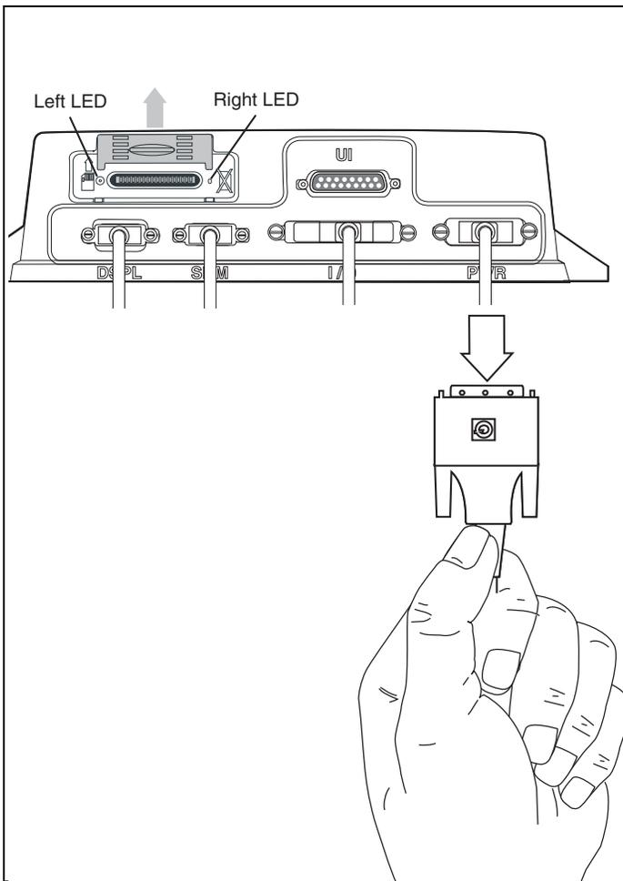
8. Reset the MAS by disconnecting the power cable. Wait for the MAS LED indicators to go out.
