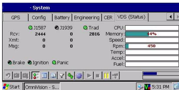
3. Verify the desired data link is enabled, as indicated by a **green LED**, on the VDS screen.
