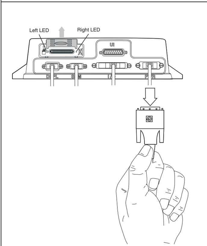
7. Reset the MAS by disconnecting the power cable. Wait for the MAS LED indicators to go out.
