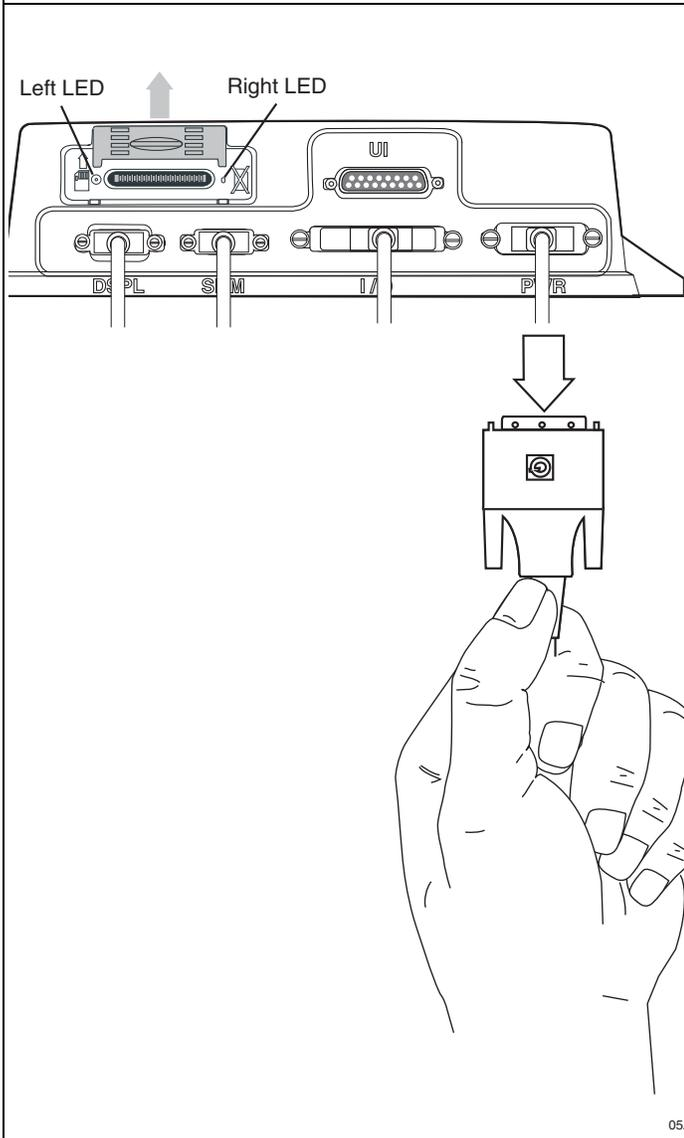
6. Reset the MAS by disconnecting the power cable. Wait for the MAS LED indicators to go out.
