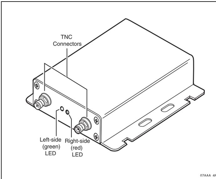
6. Test with a known good TDM. Is the left-side LED blinking green?
