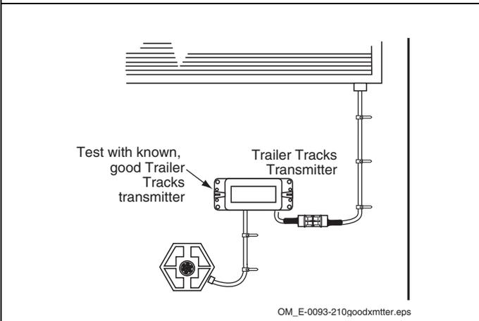
11. Check for Trailer Tracks ID with a known good Trailer Tracks transmitter.
