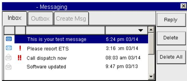
13. After a few minutes, the unit should chirp, the Message Waiting Light should come on, and a voice notification will tell you the message has been received. Tap the **Inbox** tab to display the dispatcher’s message.
