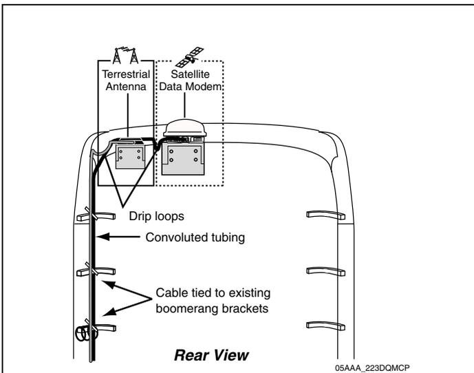
1. Make sure all cables are protected with convoluted tubing and are in good condition.
