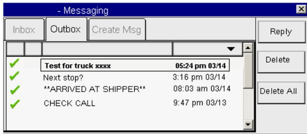
11. Tap the **Outbox** tab to display the message that was just sent. Orange “↔” (arrows) indicate the message is in transit; a green “✓” (check mark) indicates the message has been acknowledged.
