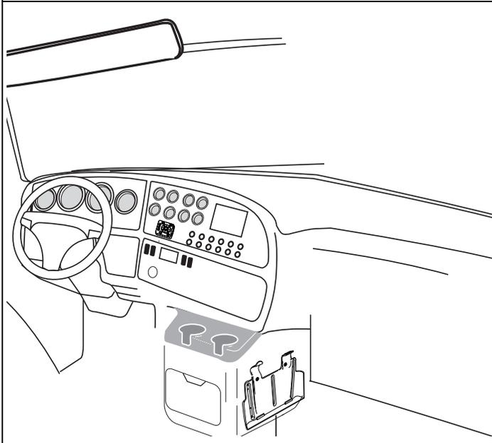
5. Make sure the display cable has enough slack and is not being rubbed or cut by anything inside the cab.
