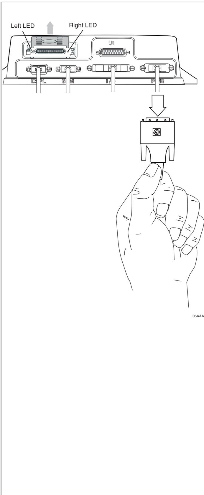
6. Reset the MAS by disconnecting the power cable. Wait for the MAS LED indicators to go out.
