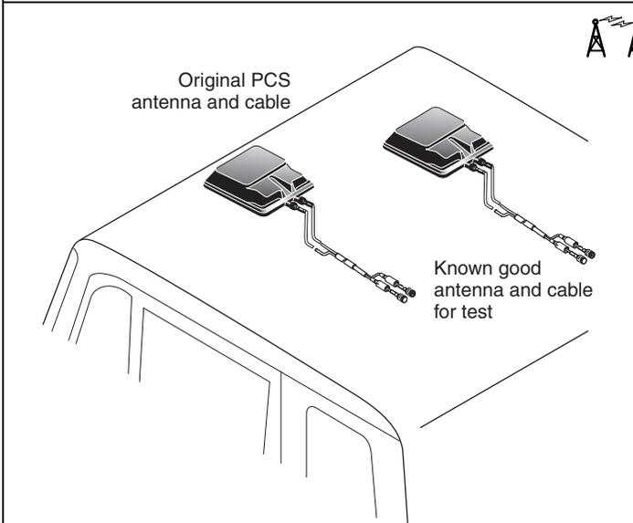
6. Test with a known good antenna and cable as follows:
