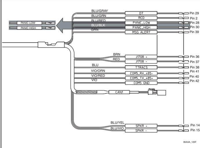
3. Using a digital voltmeter (DVM), check the resistance between pins 28 and 30 on the accessory cable connector at the MAS.
