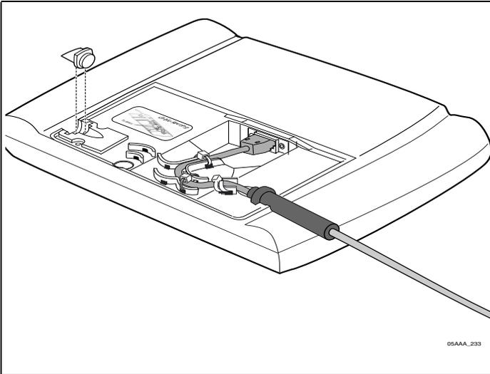
7. Inspect the underside of the MDU to make sure the tie wraps are securely tightened and the cable is not damaged.
