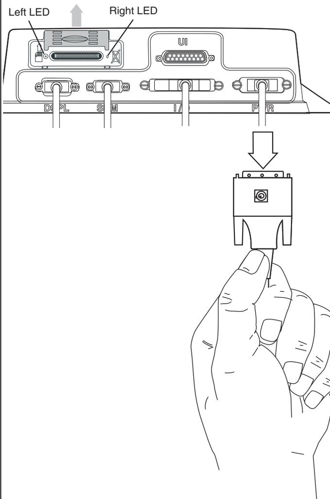
7. Reset the mobile application server (MAS) by disconnecting the power cable. Wait for the MAS LED indicators to go out.
