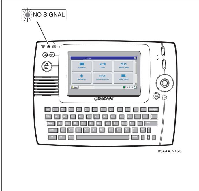
4. Check the display unit NO SIGNAL light. When the MCP100 acquires the PCS network/satellite signal, the NO SIGNAL light goes out.
