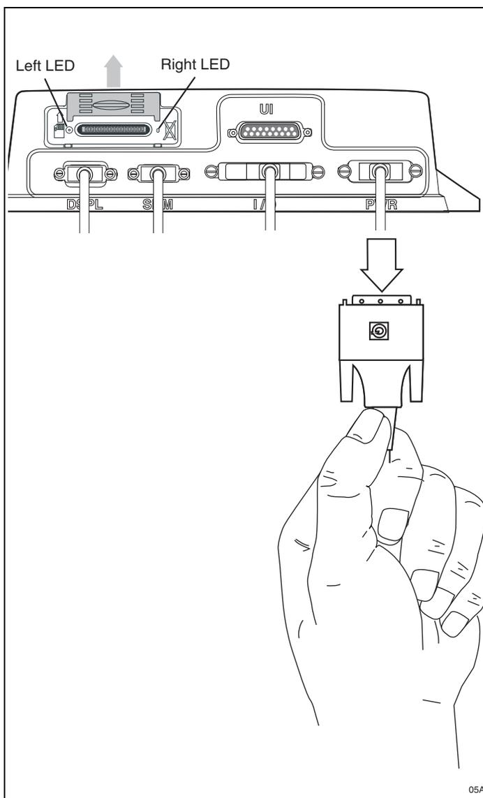
8. Reset the MAS by disconnecting the power cable. Wait for the MAS LED indicators to go out.
