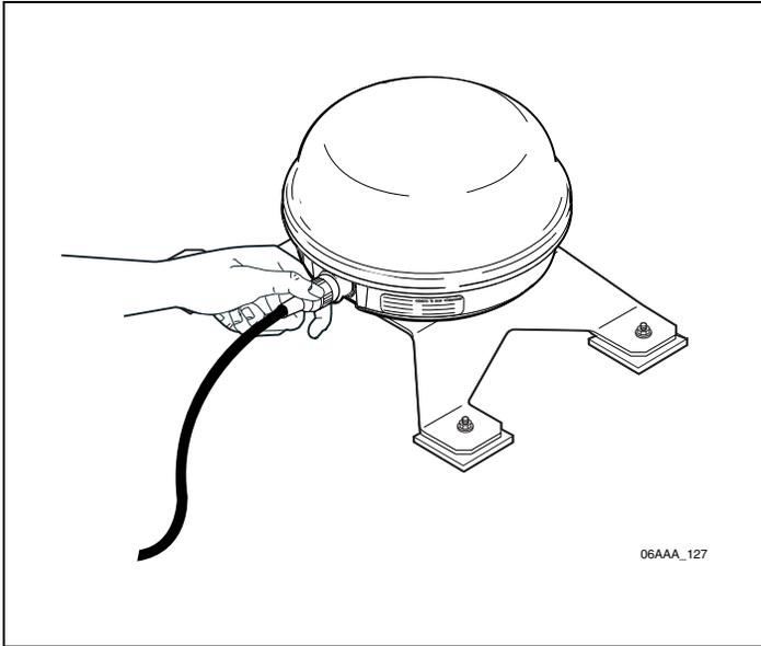
**7.** Make sure the SDM is securely attached to the SDM mount. Check the mount hardware to make sure it is secure and does not show any signs of loosening.
