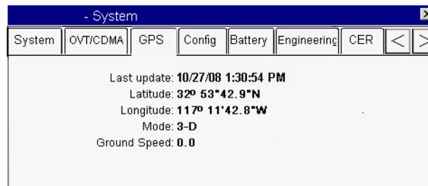
If the MCP100 is not receiving an updated position every second, shows a mode of NO FIX, or System Status 22000/22001 will not clear or reoccurs, the problem is usually caused by one or more of the following:
