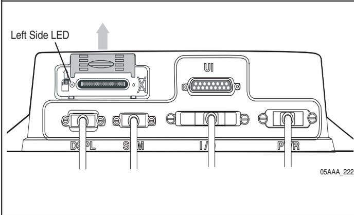
7. Check the left side LED indicator on the MAS. Normally, the left side LED indicator will be blinking blue.
