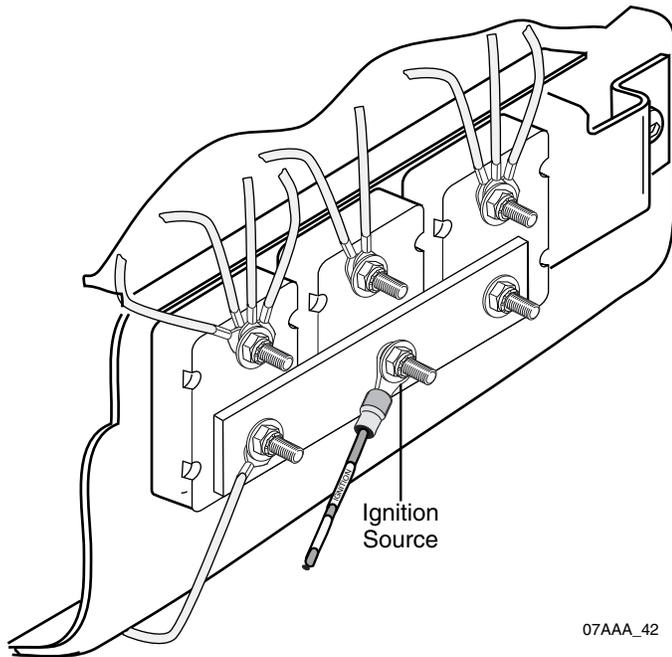
3. Check the source for the ignition wire on the vehicle. Make sure the IGNITION wire is connected to the switched +12/24 VDC power source.
