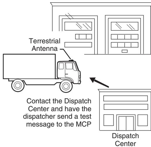
12. Have the dispatcher send a test message to the MCP100. If the dispatcher is not available, call Omnictracs Customer Support (800-541-7490) to have the message sent.
