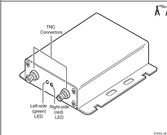
5. Check the terrestrial data modem (TDM) lights. The left-side LED should be blinking green and the right-side LED should be off.
