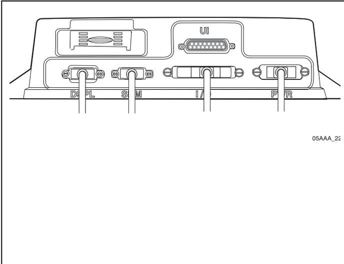
6. Make sure the cable connectors have not worked themselves loose from the MAS. Hand tighten any loose connectors.
