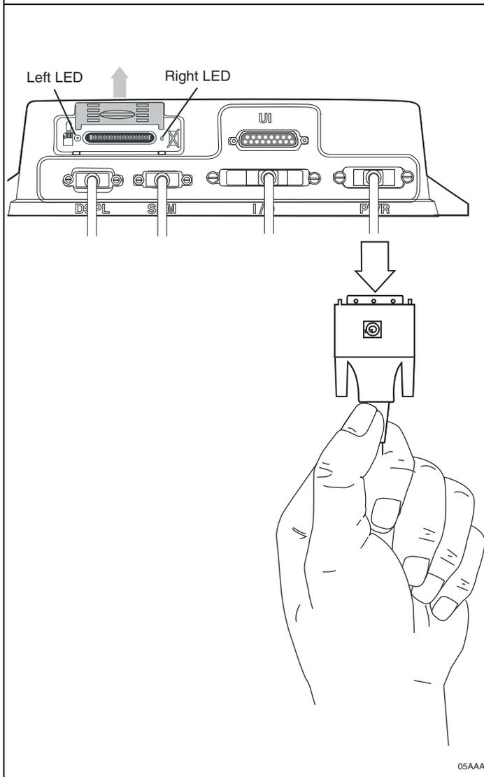
6. Reset the MAS by disconnecting the power cable. Wait for the MAS LED indicators to go out.
