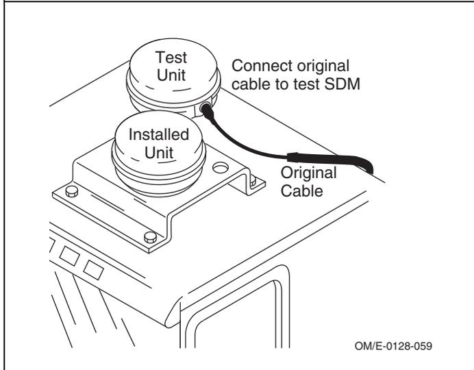
4. Connect the known good SDM. After the SDM has acquired the satellite and the NO SIGNAL light goes off, check the C/No values on the SDM screen.
