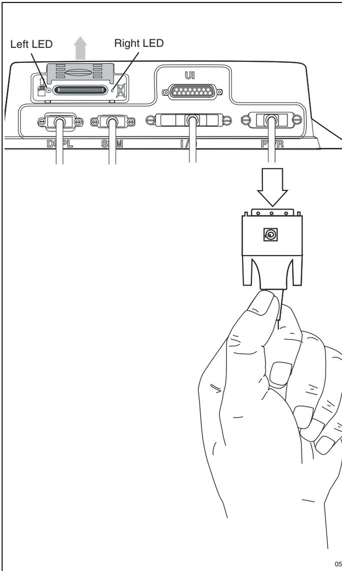
7. Reset the MAS by disconnecting the power cable. Wait for the MAS LED indicators to go out.
