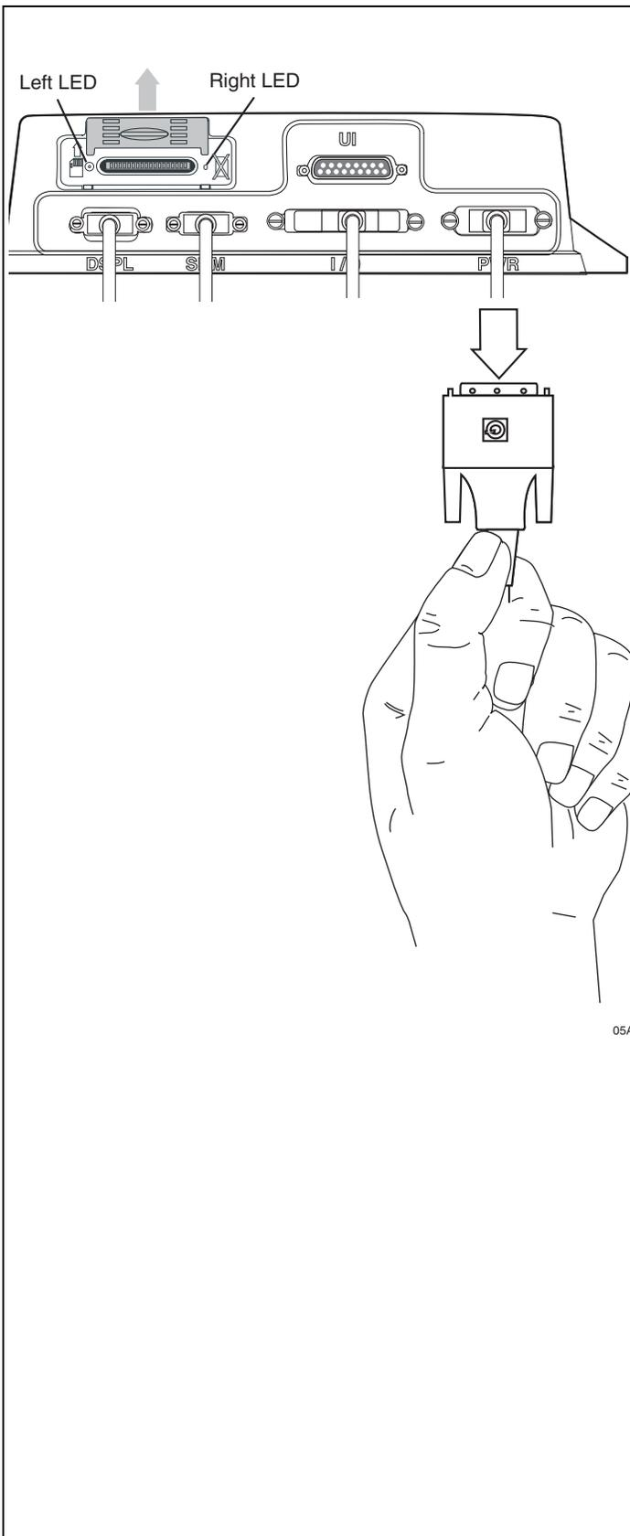
7. Reset the MAS by disconnecting the power cable. Wait for the MAS LED indicators to go out.
