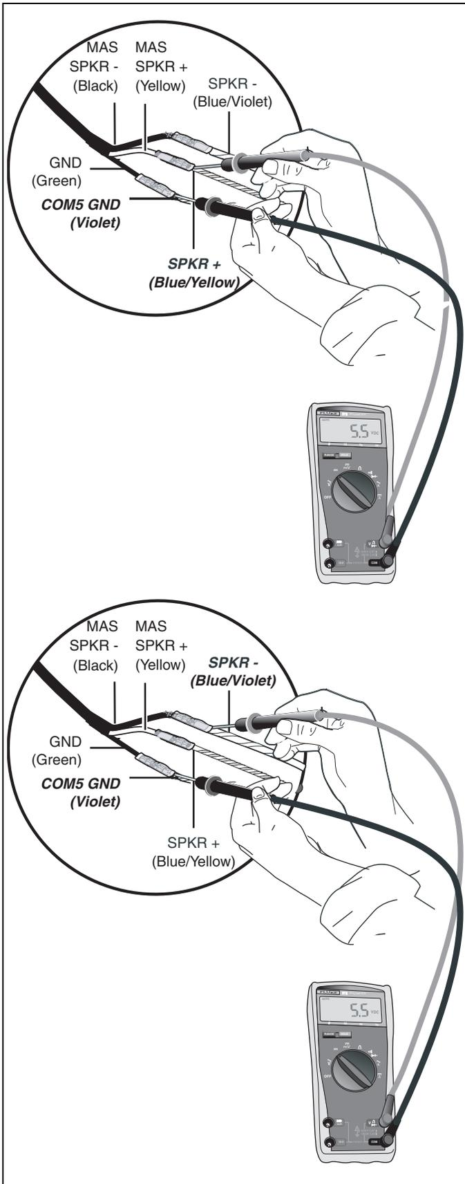
5. To isolate a problem with the speaker switch cable, measure voltages of TTS wires at end of the accessory cable, as follows.
