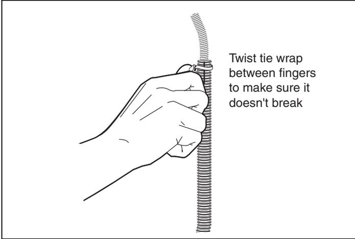
**9.** Visually inspect all tie wraps to make sure they are not brittle and do not break. If a tie wrap is damaged or brittle, replace it.
