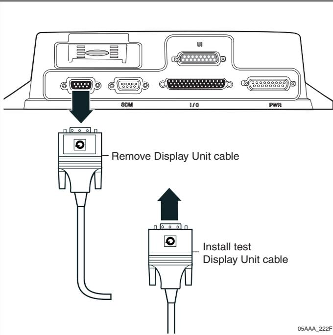
3. Reseat the display connectors on the MAS and MDU. Is the display working?
