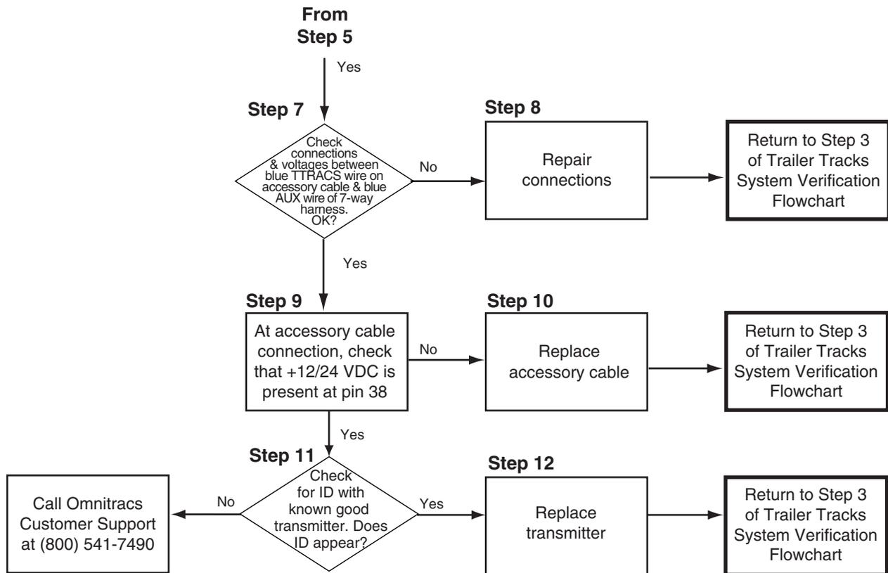
**Diagnostic Procedure A—Transmitter ID Not Displayed**
