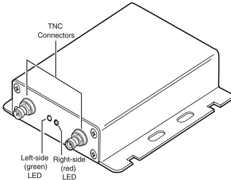
In a normal operating environment, the left side LED should be *BLINKING GREEN* and the right side LED should be *OFF*. Refer to the table below for what actions to take if the right side LED is *BLINKING RED*.
