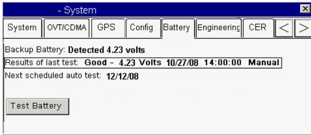
10. Go to the Home screen and tap the **System** icon. Tap the **Battery** tab and tap the **Test Battery** button.
