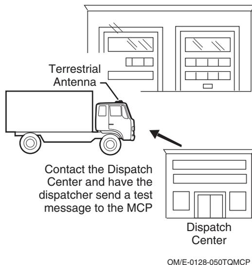
8. Contact the dispatcher and verify that the MCP100 unit address listed on the MAS matches the number listed for this vehicle in the MCP100# field of the host software.
