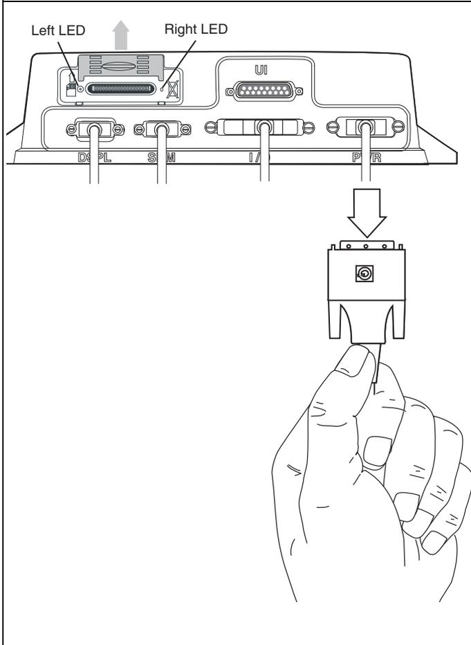
5. Reset the MAS by disconnecting the power cable. Wait for the MAS LED indicators to go out.
