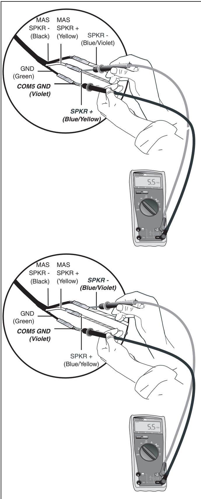
6. To isolate a problem with the speaker switch cable, measure voltages of TTS wires at end of the accessory cable, as follows:
