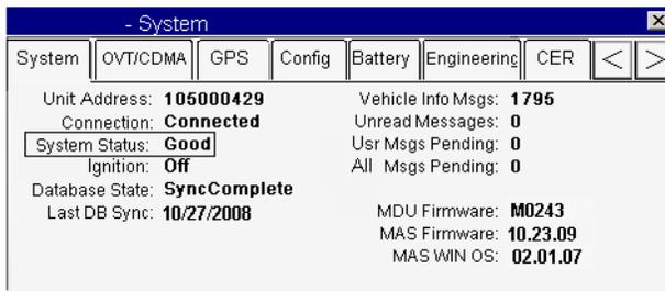
When vehicle ignition is turned OFF, the System Status should change to **Ignition Off** within 10 minutes.
