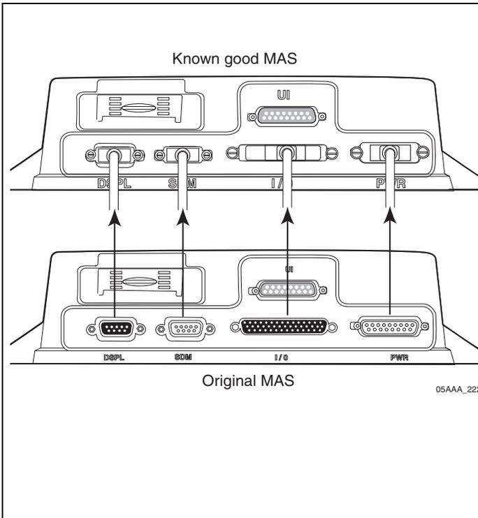
8. Replace the original MAS with a known good MAS. Is the RCD functioning and can you hear the announcement?
