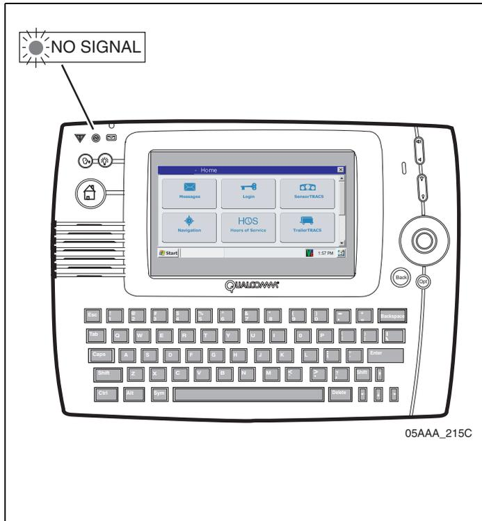
3. Check the NO SIGNAL light on the display. After the MCP100 acquires the satellite, the NO SIGNAL light will go off.
