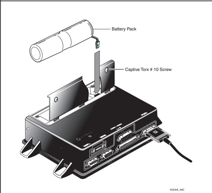
2. Install a new battery into the MAS.
