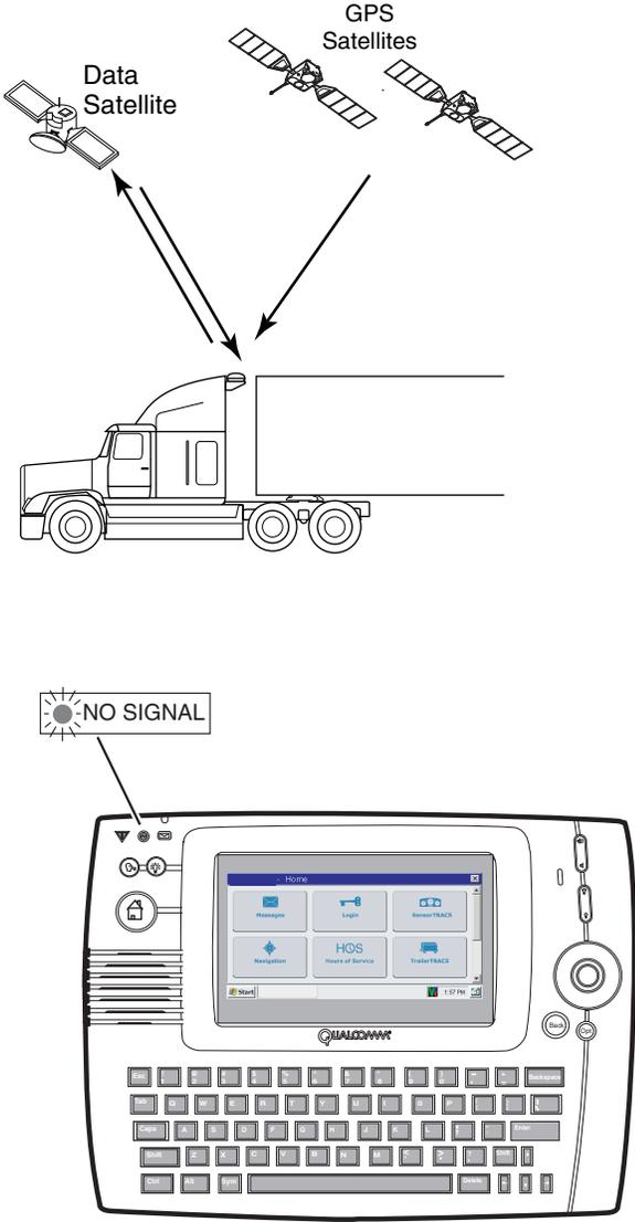
The diagram illustrates the diagnostic procedure for a low satellite signal. It shows a truck receiving signals from a Data Satellite and GPS Satellites. Below the truck is a close-up of the MCP100 device with a 'NO SIGNAL' warning icon pointing to the top left corner of the screen.
