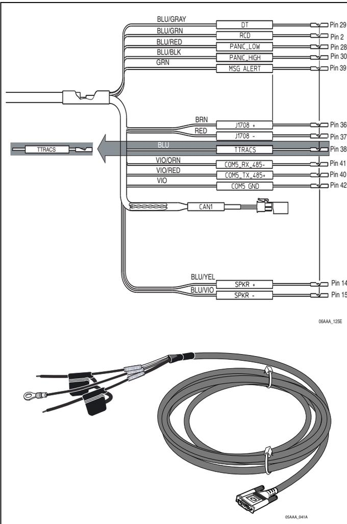
9. At the accessory cable, check that +12/24 VDC is present at pin 38 and using chassis ground.
