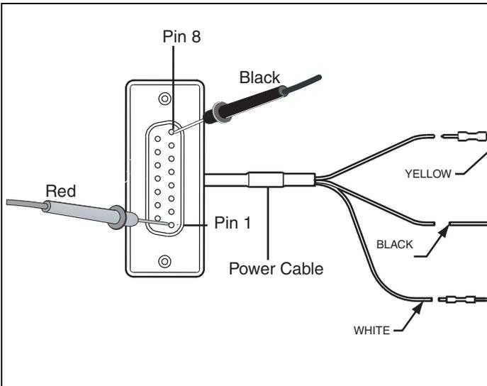
5. Check the MAS power cable connections. Is BAT+ connected to an unswitched +12/24 VDC constant power source? Is IGN connected to a switched +12/24 VDC power source?
