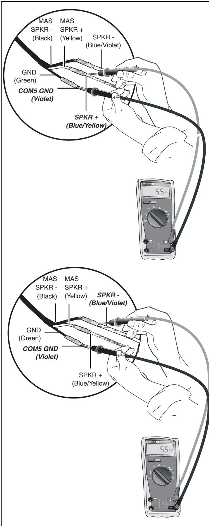
11. To isolate a problem with the speaker switch cable, measure voltages of TTS wires at end of the accessory cable, as follows:
