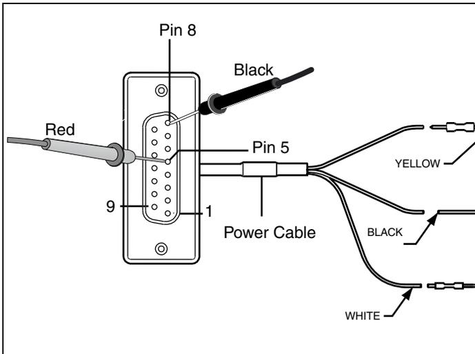
4. Disconnect the power cable from the MAS. Use a voltmeter to test pin 5, as follows:
