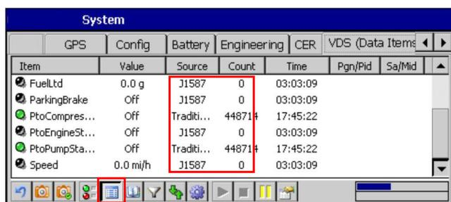
3. Check the VDS Configuration/Ports screen. Does the VDS configuration match the hardware configuration (CAN1 or CAN0 only)?
