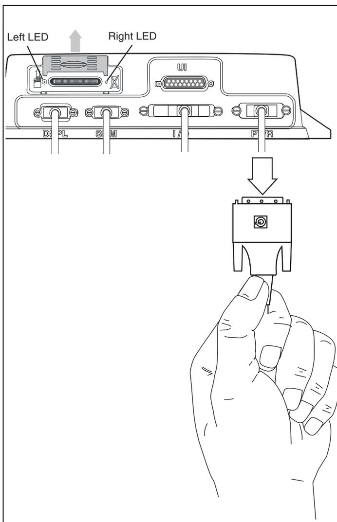
3. Reset the MAS by disconnecting the power cable. Wait for the MAS LED indicators to go out.
