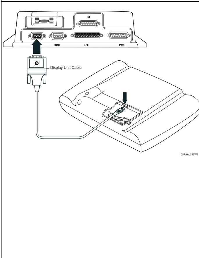
3. Reseat the display connectors on the MAS and MDU. Has the Loading screen cleared?
