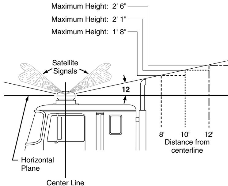
An obstruction height of 2.5 feet for every 12 feet away from the SDM centerline is acceptable. The MCP100 may not operate properly if there are obstructions above this height. Use this same formula to verify that a trailer hooked up to the vehicle does not extend above the 12° angle.
