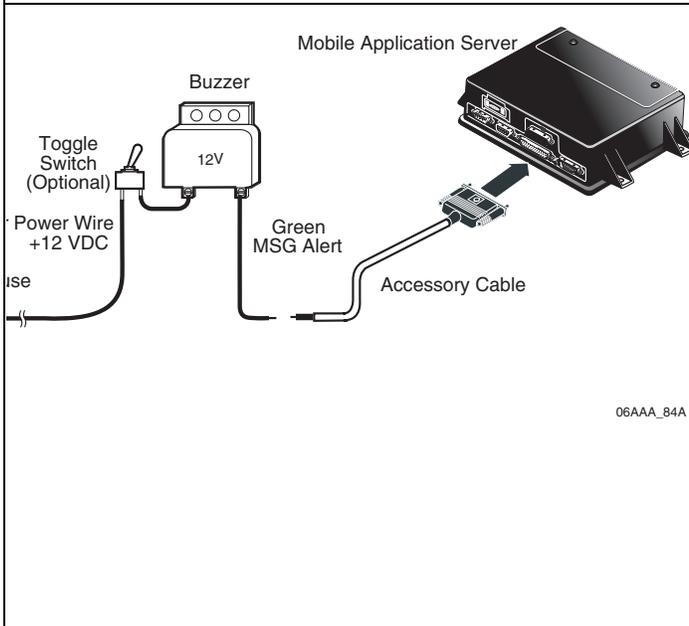
**5. Disconnect the buzzer/RMWL wiring from the accessory cable's green MSG ALERT wire. Is the buzzer/RMWL on or off?**
