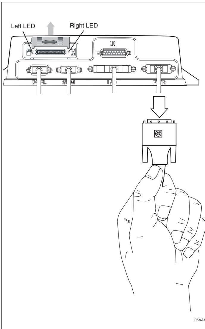
7. Reset the MAS by disconnecting the power cable. Wait for the MAS LED indicators to go out.
