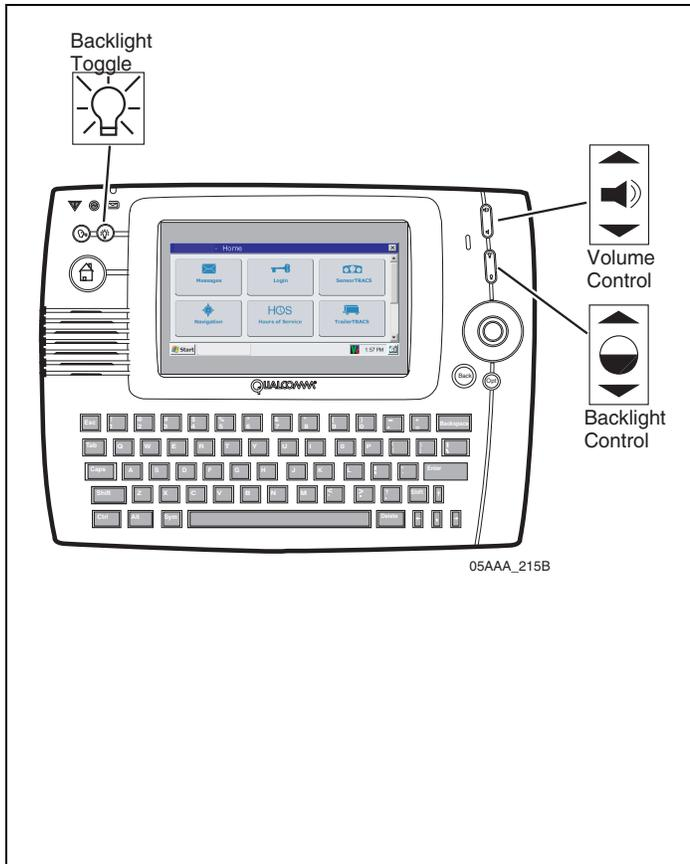
3. Check the display unit and verify that the screen lights up and displays characters; and that the backlight, brightness, and volume controls work correctly.
