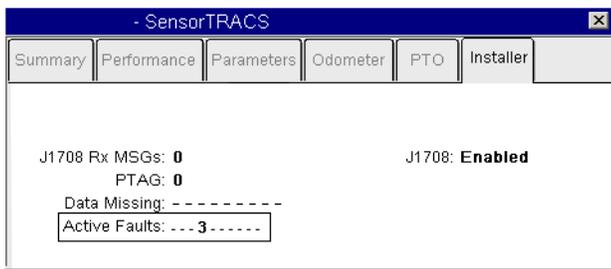
6. Check that an ACTIVE FAULTS number is present. Refer to **Data Missing Indicators and Active Fault Values** on page 21-7 for specific information.
