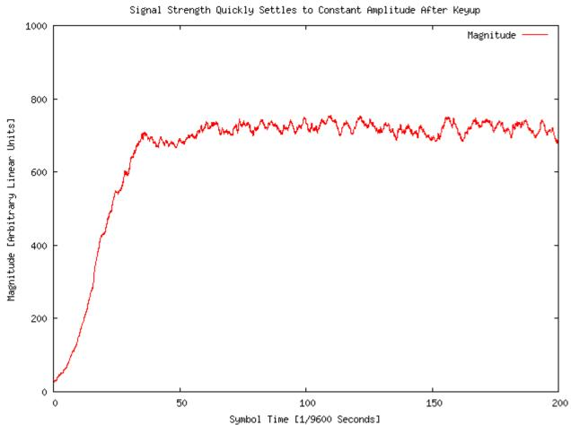
Illustration 4: Signal envelope starting from transmitter keyup at approximately time zero. Power ramps up within three milliseconds. Filtered with approximately 500  $\mu$ S time constant.
