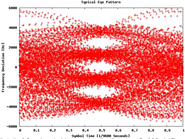
Illustration 6: Example received data eye pattern. Sampling occurs at T = 0.5 Symbol Times. The eye has opened adequately at the expected sample time and we expect a symbol stream with few errors. Note: Final RRC filter not applied, moderate S/N.
