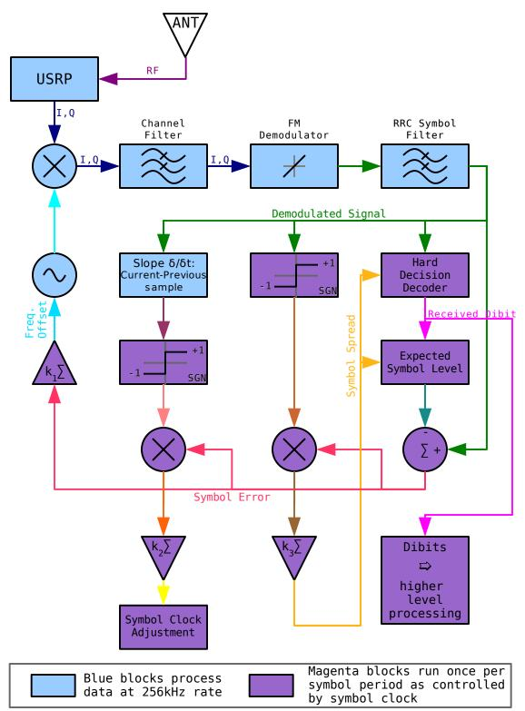
Drawing 1: Four Level FSK receiver block diagram. k1, k2, and k3 constants set frequency offset, symbol clock, and symbol spread (carrier deviation) sensitivity respectively. Not shown: hard limits on symbol spread and frequency offset adjustment ranges.
