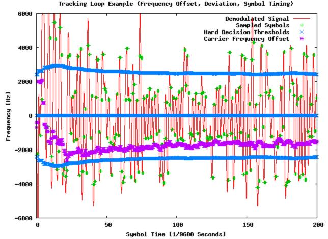
Illustration 5: Four level FSK symbol recovery showing successful carrier tracking of the 859.7375MHz Burritt Museum Transmitter Site Signal. Transmitter key up has occurred around time zero. Acquisition has succeeded by about the 25th symbol time point. Note the atrocious carrier frequency drift which can exceed 1 kHz over the medium term (order of seconds)!
