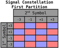
Table 4: First partition of constellation using redundant error correction bit.The two partitions are shown colored in salmon and violet.(Apologies to the salmon/violet colorblind).
