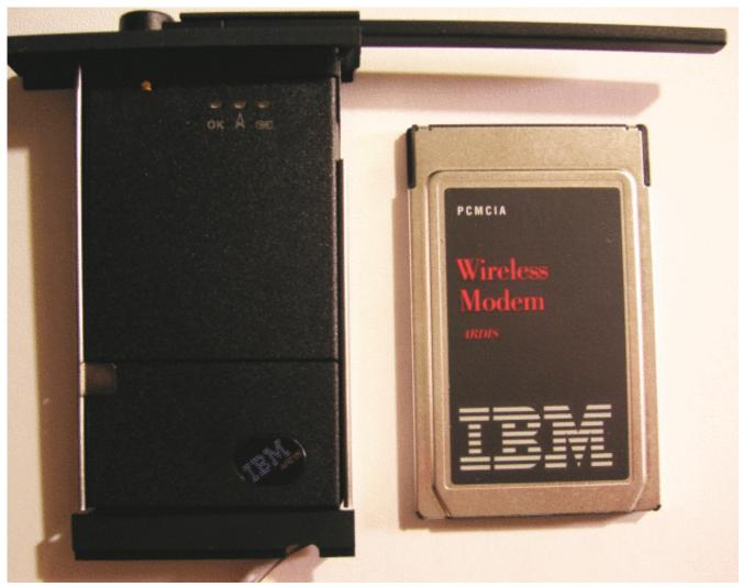
Illustration 1: Surplus 90's vintage 19,200 bps RD-LAP PCMCIA wireless modem card with antenna adapter. Frequency coverage of 806-825, 851-870 MHz perfectly matches public safety systems.
