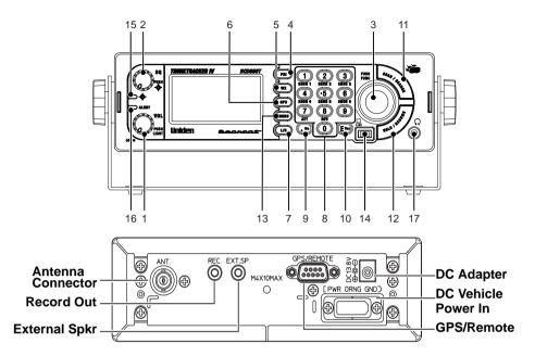
The knobs and keys on the BCD996T produce several different actions. You can, for example, rotate the knobs as well as press them to achieve a different result. Pressing a key briefly can produce one result while pressing and holding, gives a different result.
