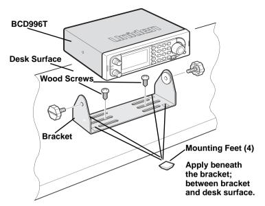
To secure the radio, by means of the mounting bracket, to a surface, follow the steps below:
