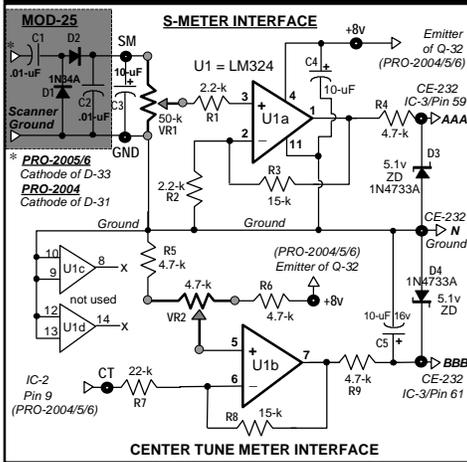
You can increase R3 or decrease R2 for more gain, as needed. If R2 is increased to 3.3-k, the gain drops to **4.5**; 4.7-k drops the gain even more to **3.2**. A lot depends on the output of the S-meter circuit at max signal input. If a walkie talkie held near the scanner results in an output at the top of VR1 of 0.6v, then to get the full 5v limit out of U1a, you'd need a gain of  $(\frac{5}{0.6}) = \mathbf{8.3}$  in which case R2 should be about 1.8-k.
