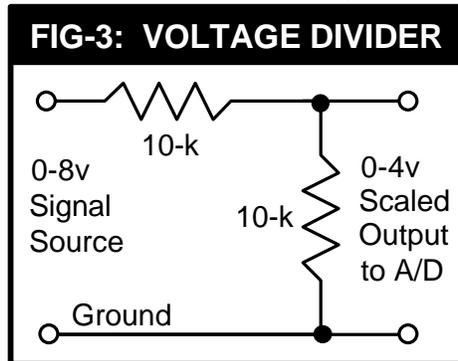
recalculates it back to 4 volts. You need only remember the scaling factor, in this
