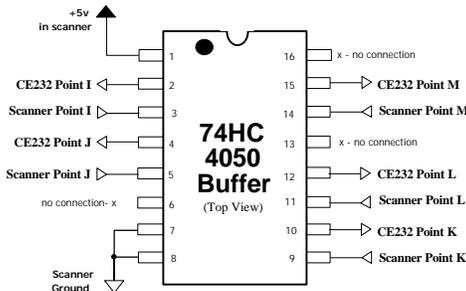
Install this circuit as close as possible to Points I, J, K, L, & M on the scanner's Logic/CPU Board. (Scanner "Points" are on the Logic/CPU Board. CE-232 "Points" are on the HB/CE-232 Board.)
