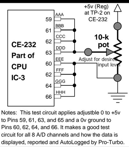
Notes: This test circuit applies adjustable 0 to +5v to Pins 59, 61, 63, and 65 and a 0v ground to Pins 60, 62, 64, and 66. It makes a good test circuit for all 8 A/D channels and how the data is displayed, reported and AutoLogged by Pro-Turbo.
