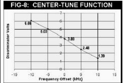
Connect the "CT" point on the A/D Signal Conditioner board to IC-2/Pin-9 in the scanner and have a voltmeter connected to Point BBB. Repeat the above test for off-frequency signals and take your own data like I did. You'll get similar results.
