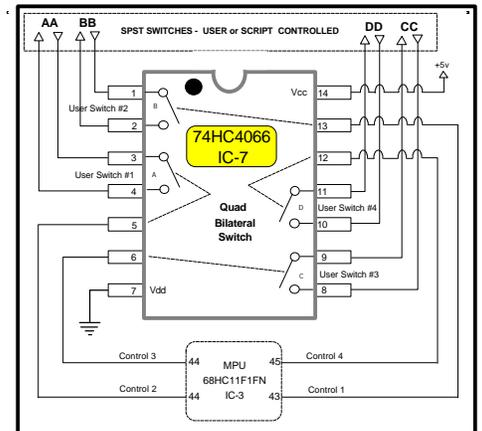
Another of the HB/CE-232's claims to fame is the 6-bits of *read-only* ports that we call the *Status Inputs*. In a word, when we designed the HB/CE-232, we couldn't figure out what to do with the spare input ports of the powerful microprocessor that runs the interface. So we allocated six of
