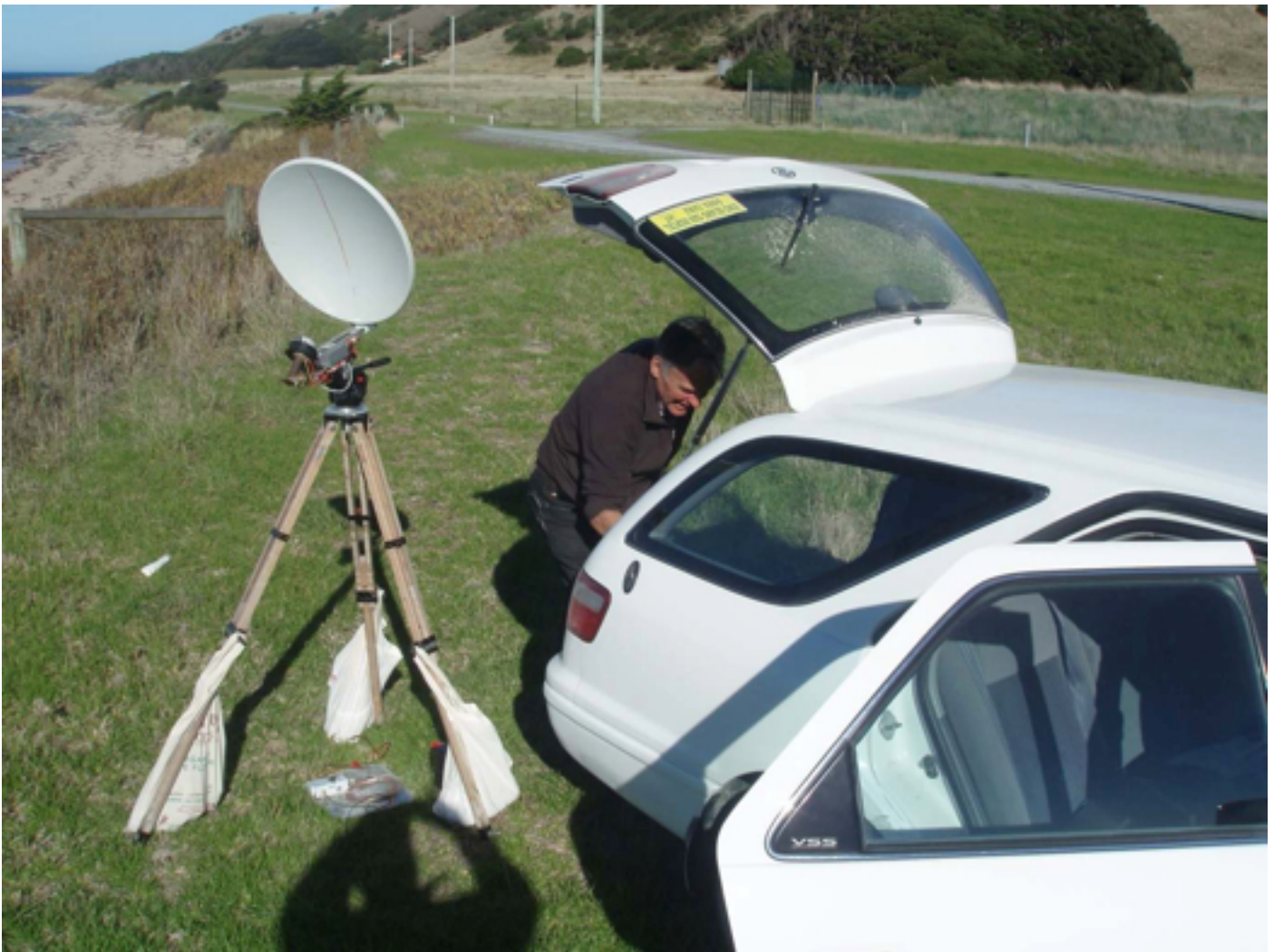
Fig 3: 10 GHz system at QF20, tripod stabilized with shopping bags full of rocks
