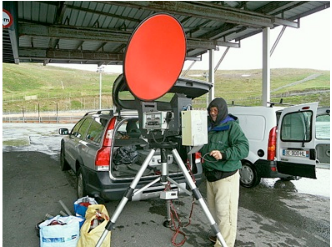
The 24GHz rig in the shelter of a service station, due to bad wx and is taken from F1FIH webpage http://f1fih.over-blog.com/pags/C37SHF_2012-7910566.html
