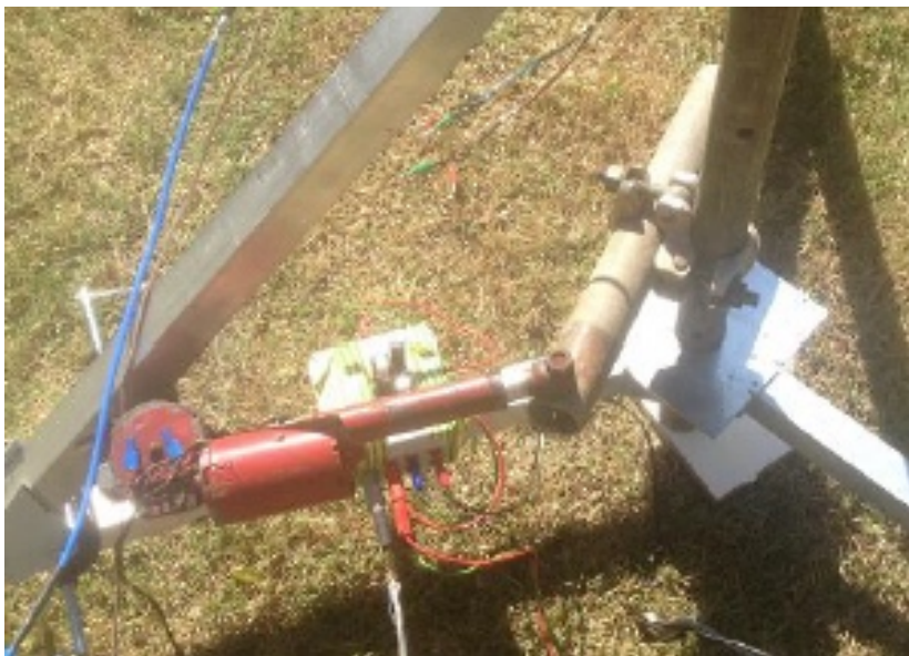
Azimuth actuator giving about 50 deg of movement.
