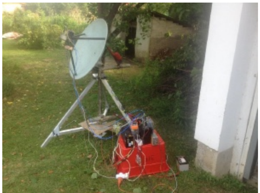
Complete system. 10GHz transverter + LO, power supplies etc on top of box.
