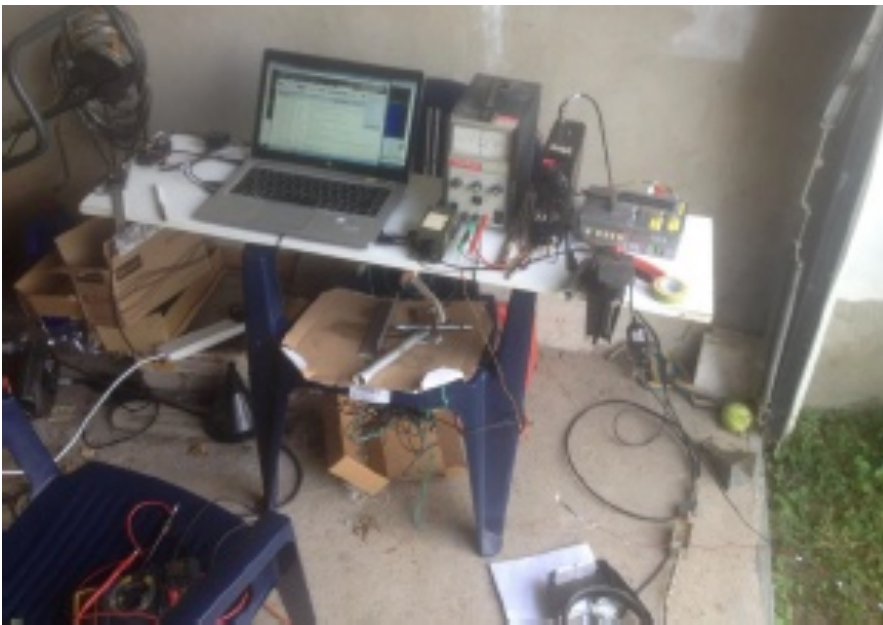
Operating position showing PC, Morse key, PSU, IC202 and SDR
