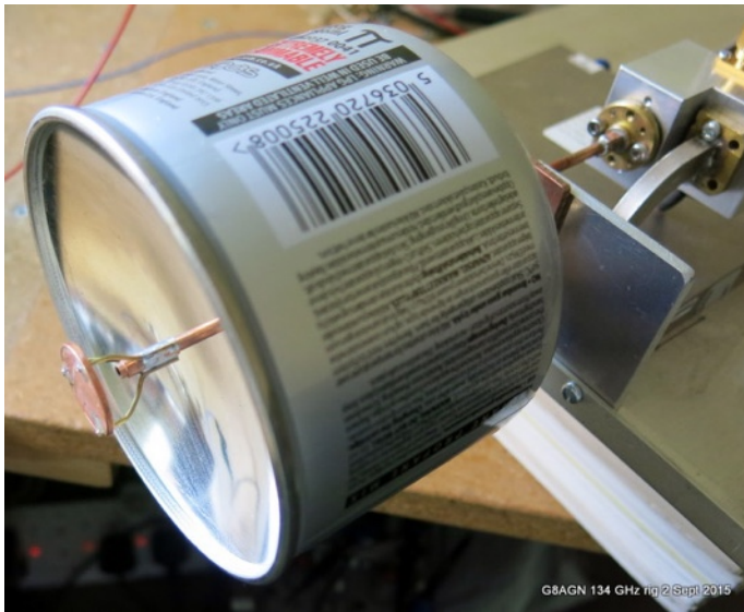
Photo 3: New penny feed fitted to the gas canister dish
