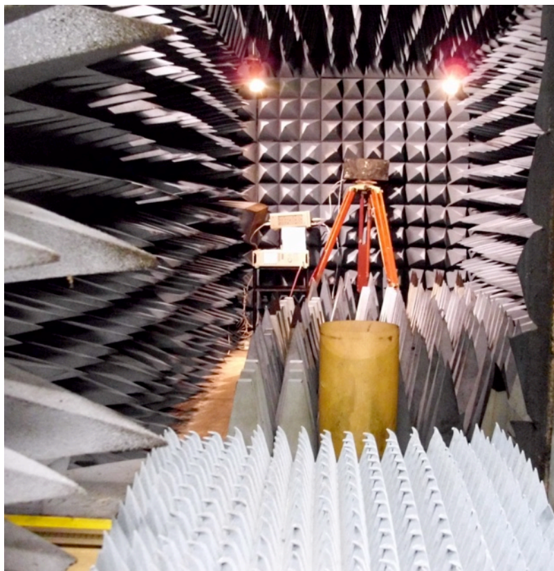
8 Metre test range using anechoic chamber and control room to get the distance
