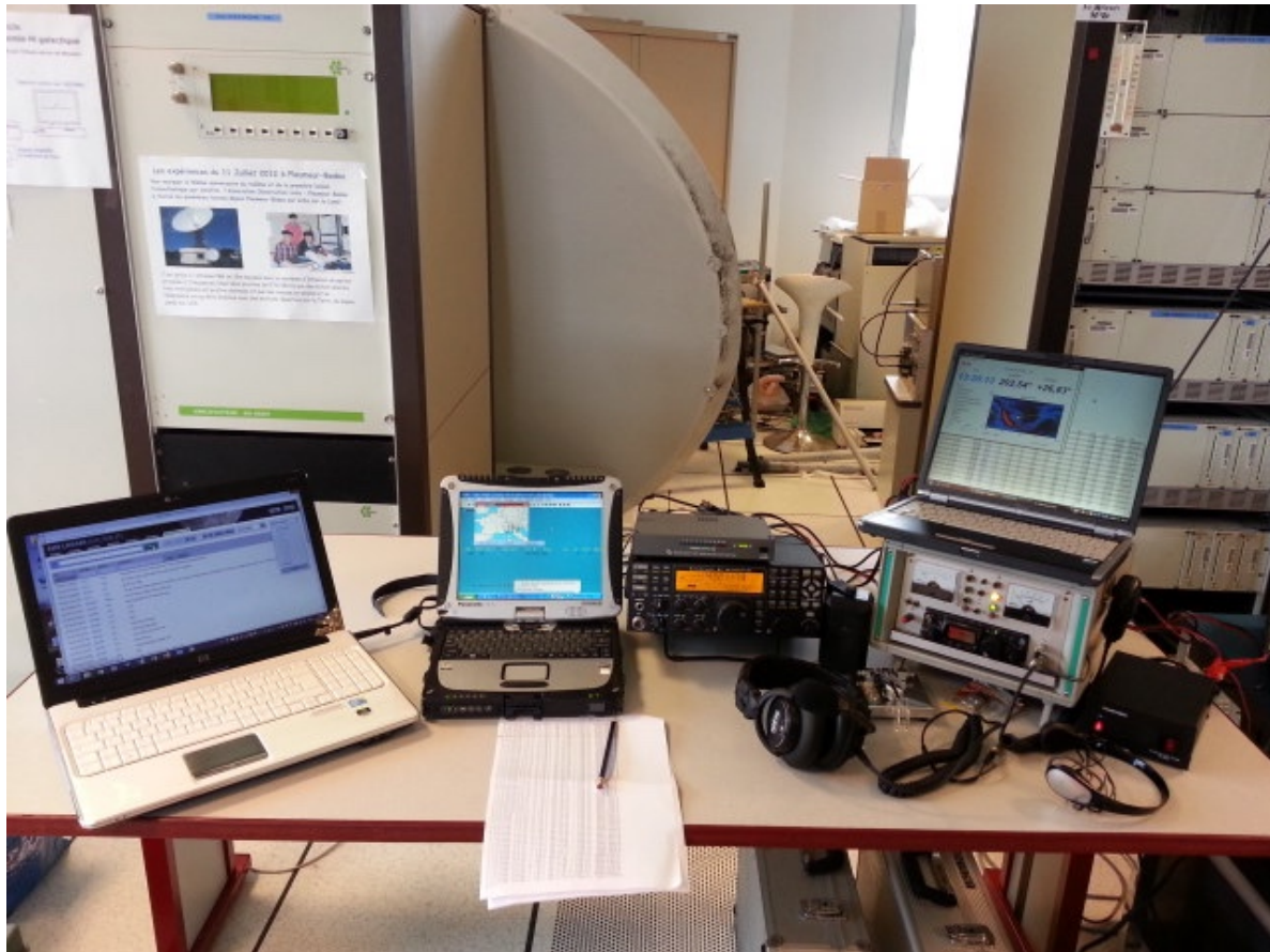
K3 + 432/28MHz tvt + Doppler shift compensation
