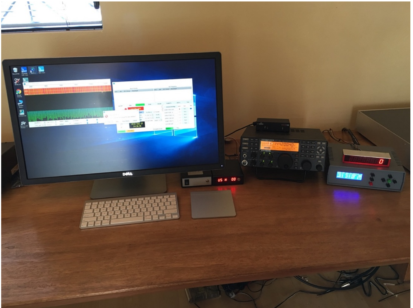
Left to right: sequencer, polarization controller, K3 ( w/ SDR-IQ above it), OE5JFL controller (with remote SSPA power monitor above it)
