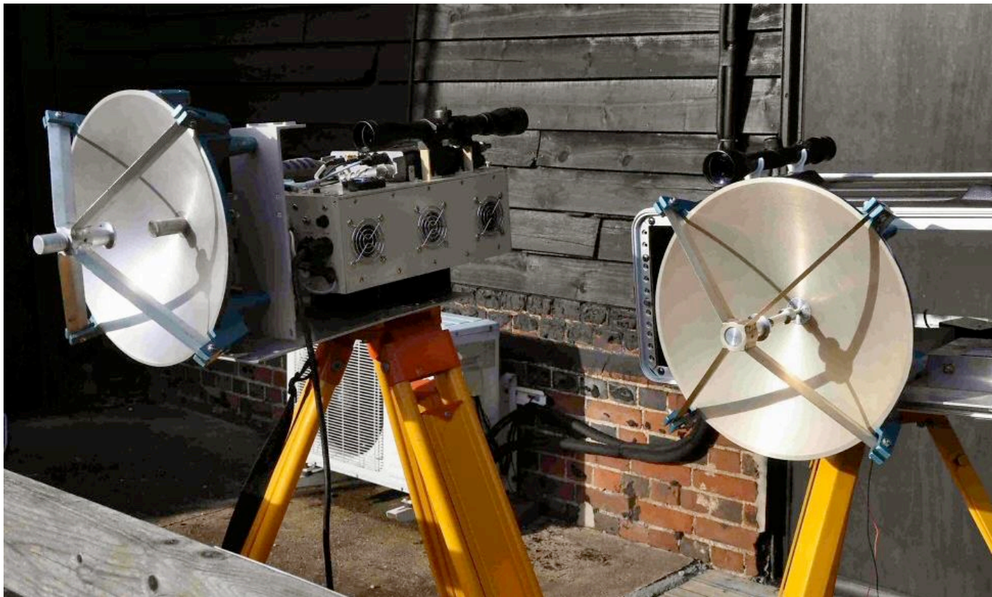
Figure 1: 241 GHz Transverters for the first UK 241 GHz QSOs. Source: Scatterpoint March 2016
