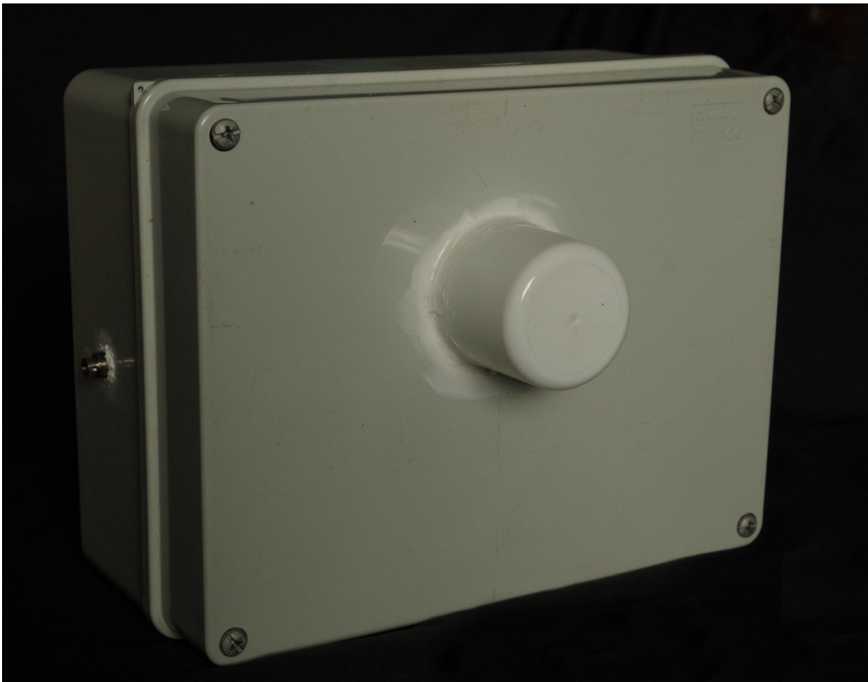
Photo 3 External view showing the Radome glued in place. The connector on the side carries the 12V DC input
