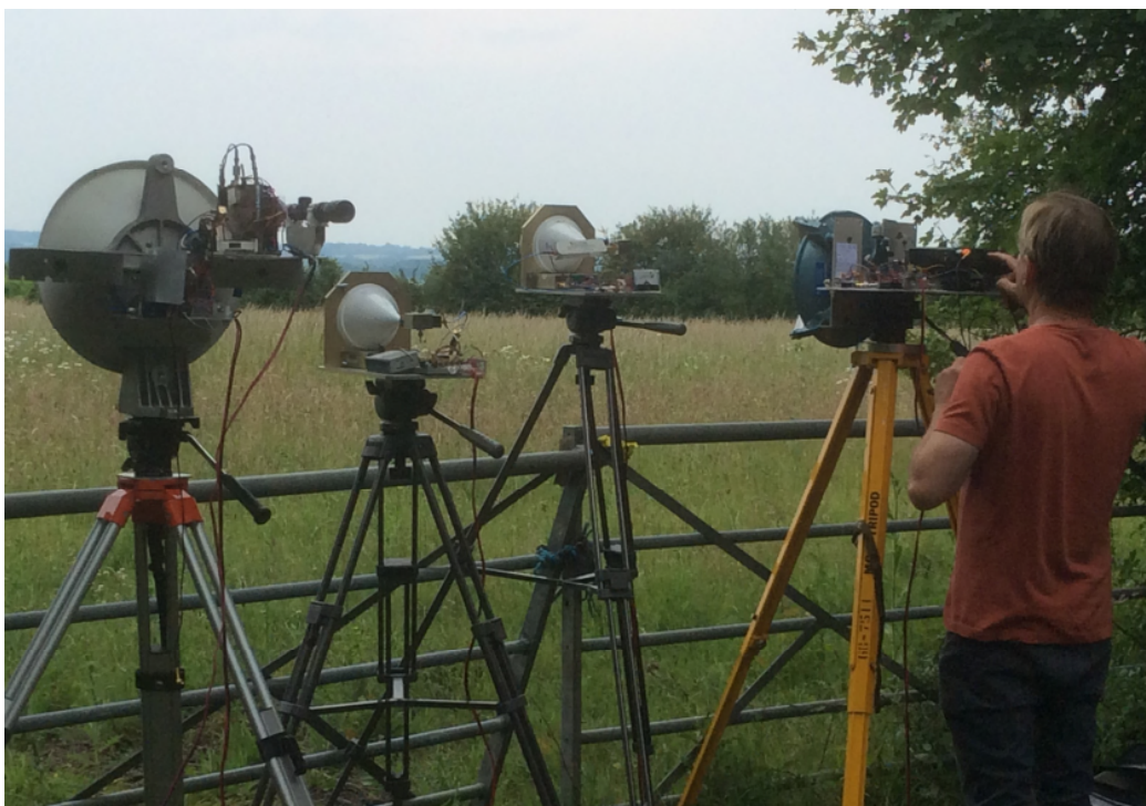
G8CUB at Shroner Wood left to right 241G RX, 241 TX, 134 TX, 134 RX
