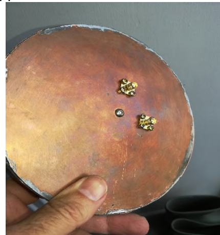
Photo 5: SM6FHZ patch (after filing) showing rear with SMA sockets
