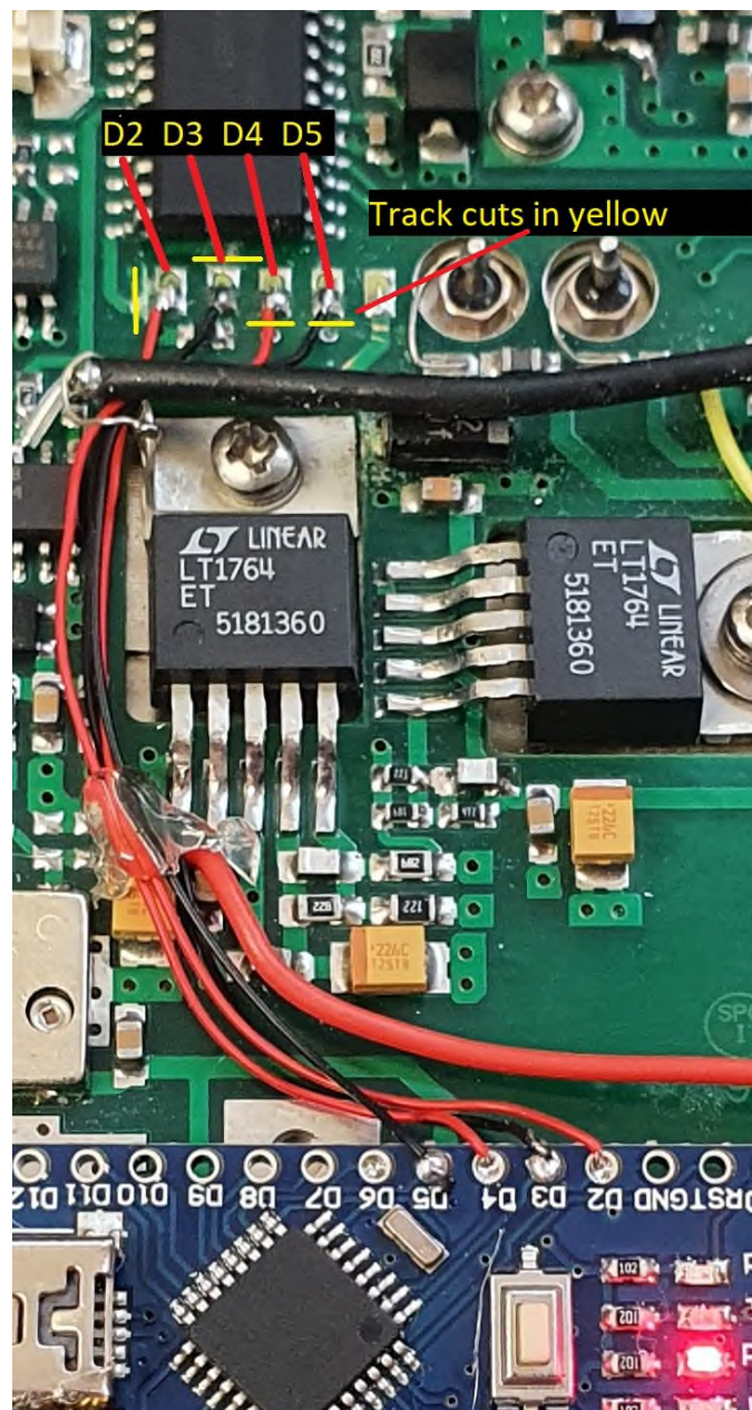
Photo 5 Track cuts on the Elcom and connections to the Arduino
