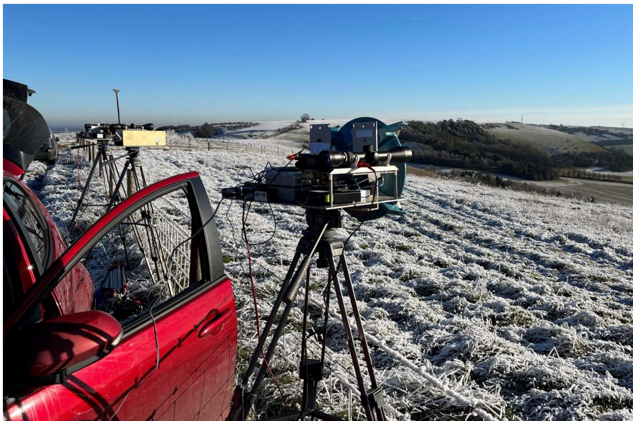
From right to left. 122/134 tx/rx 30cm dish, 25mW 122 beacon 150mm horn, second 122 system 100m lens horns
