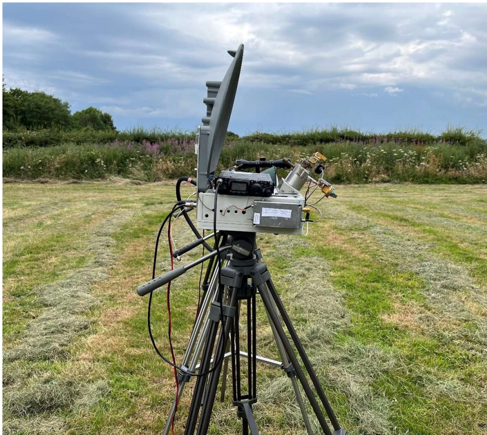
G8CUB - Testing 47GHz transverter front, and 76GHz transverter rear on receive to use the next day.
