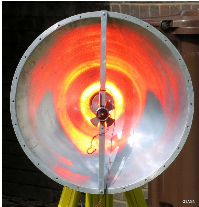
Figure 2: Here the MCH heater has been swapped with a 3W red LED for dish alignment
