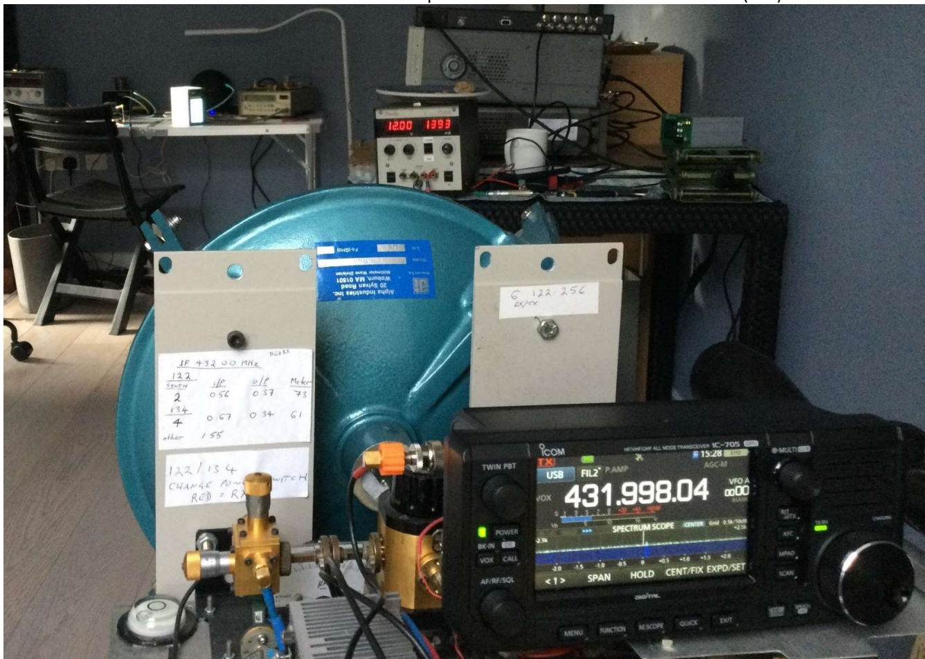
The 8GHz signal generator is on table sat vertically @ 30 degrees for best output at this frequency.
