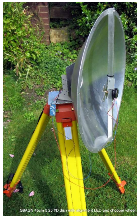
Figure 1: MCH heater and chopper wheel placed at dish focus
