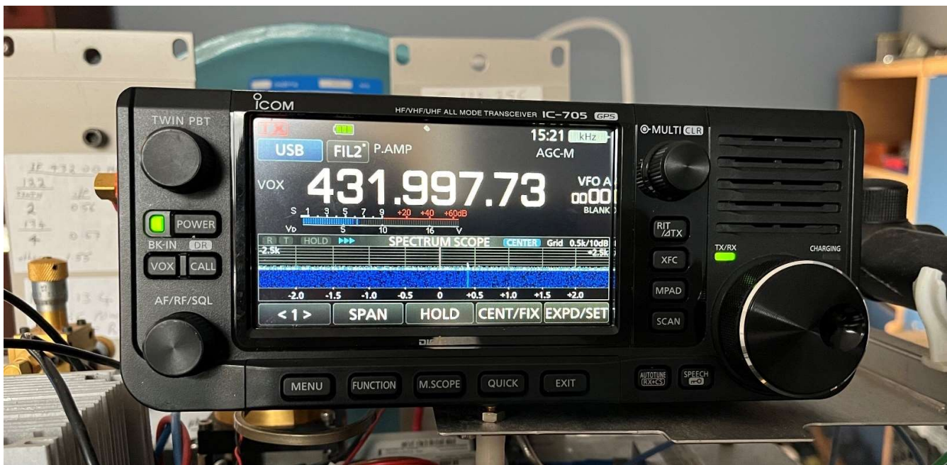
122.4GHz harmonic received at 3 metres. Line on the spectrum can be seen between 0 and 0.5 (kHz)
