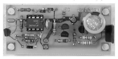
Glue, or use a dab of heat sink compound and clamp it on. A heat sink takes some time to heat and cool, so the fan will not change speed instantaneously, but will speed up as the heat sink heats. More important, it will continue running at higher speed until it brings the heat sink temperature down, gracefully slowing down as things cool. U2 need not be mounted on the printed circuit board, but may be mounted remotely, on the heat sink; twist the wires together, and
