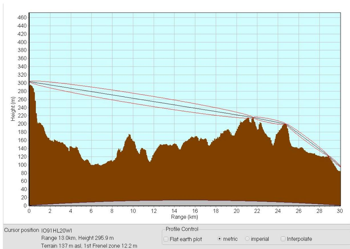
The profile shows the earth bulge corrected for the effective earth radius based on the value in the K-Factor box. Usually a 4/3 effective earth radius is used. In order to see the terrain for longer paths, there is an option to flatten out the earth bulge - this is only a visual aid and has no effect on the profiles.
