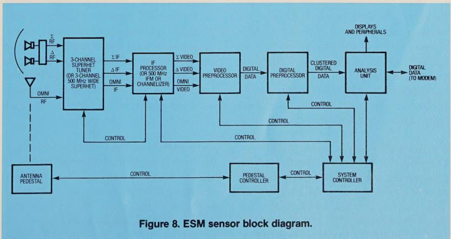
Figure 8. ESM sensor block diagram.
