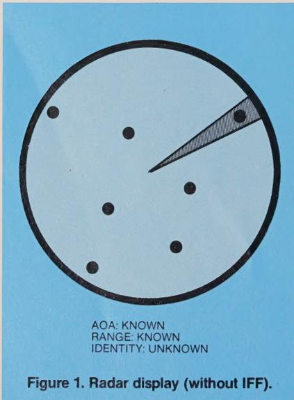
Figure 1. Radar display (without IFF).
