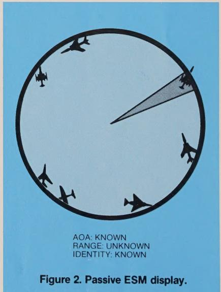
Figure 2. Passive ESM display.
