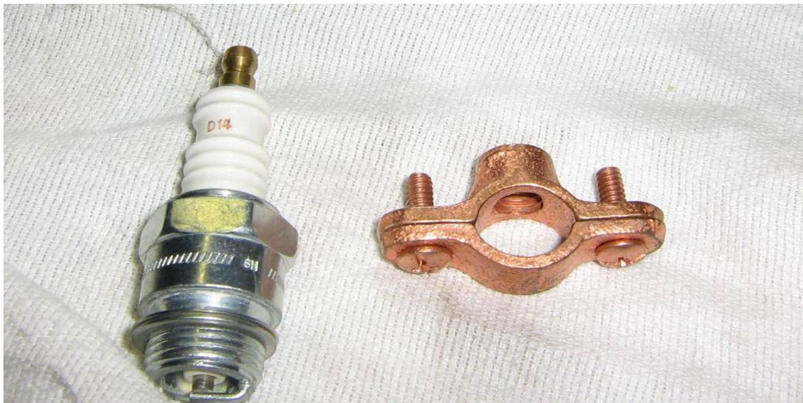
An automotive spark plug will be used for the spark gap. A Champion D14 is shown here. Be sure it *doesn't* have an internal resistor. A copper pipe ground clamp will be used to hold the spark plug, which will then be attached to the side of the magnetron's case.
