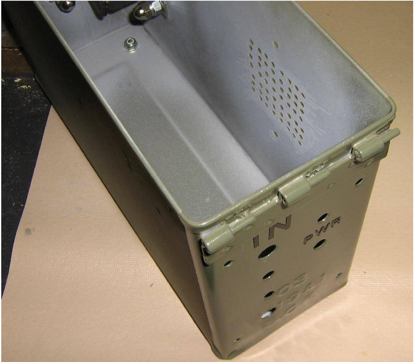
Alternate view showing the front-panel and the array of 1/8-inch diameter speaker holes. In the rear, two L-brackets secure the battery pack to the side of the case. The holes on the left side of the front-panel are for a 1/4-inch jack, a 1/8-inch jack, a RCA jack, and a BNC jack.
