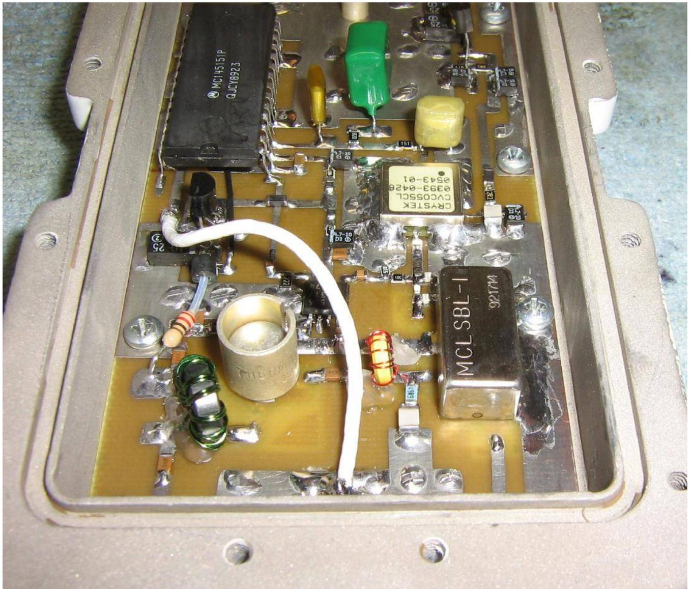
The 445 MHz local oscillator is created by a PLL frequency synthesizer circuit using a Motorola MC145151 synthesizer IC and a Crystek CVCO55CL-0393-0428 Voltage Controlled Oscillator (VCO).
