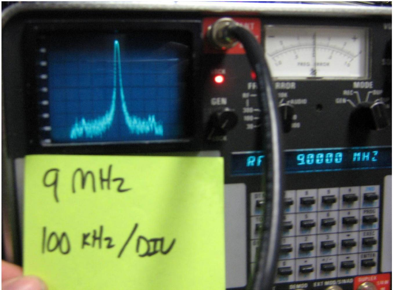
Spectrum analyzer view of the 9 MHz second IF output with a  $-30$  dBm 436 MHz RF input signal.
