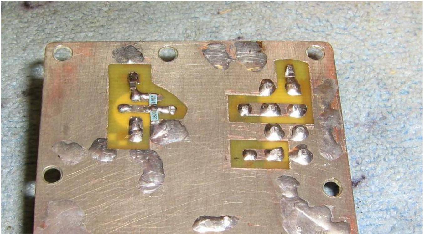
The PC board was made via a "psuedo double-sided" technique.
