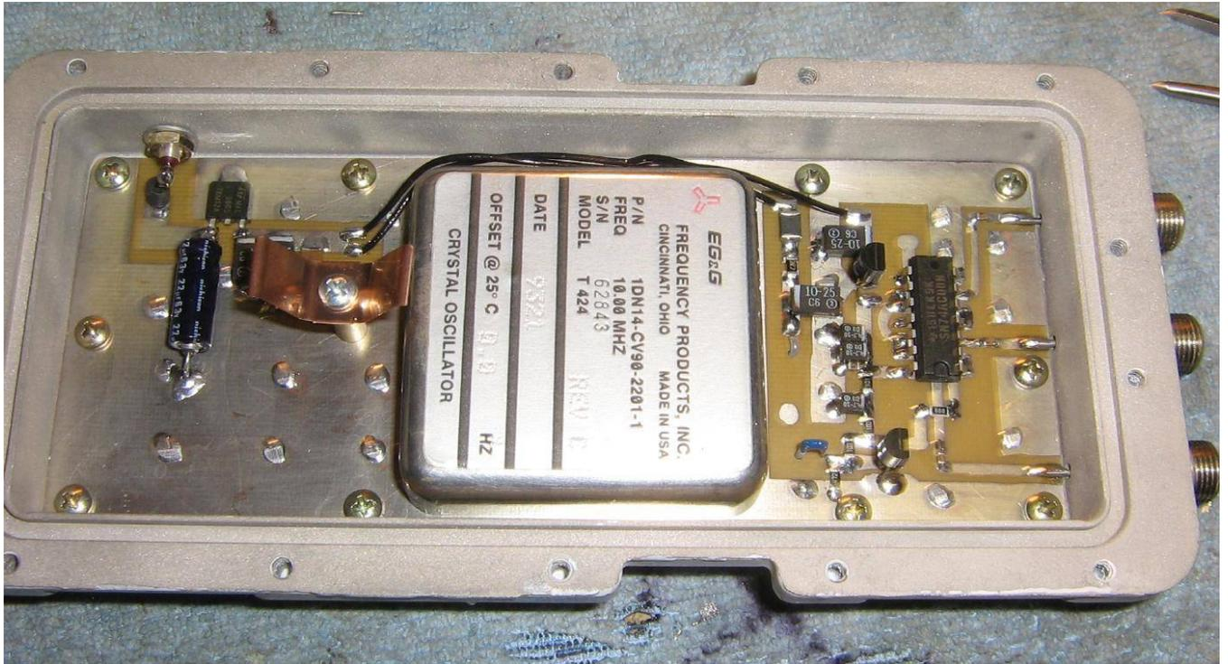
10 MHz Temperature Compensated Crystal Oscillator (TCXO) time base.
