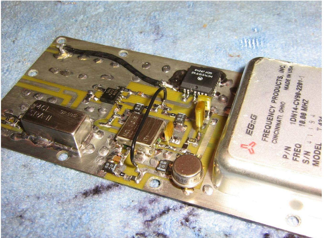
Closeup view of the PLL and VCO sections.
