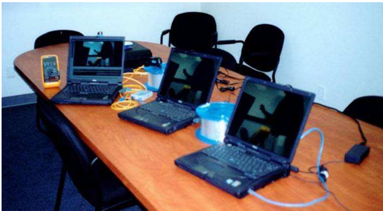
3(e). Example of the tapping of a live video conference over a 10 kilometer fiber span without network disruption or visible signal degradation in a laboratory setting. Intercepted video conference between two laptops replayed on third laptop in real-time.
